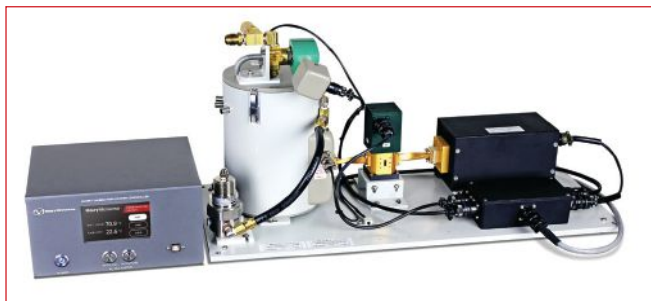
▲ Fig. 2 Noise calibration system with reference termination immersed in liquid nitrogen. Source: Maury Microwave.
