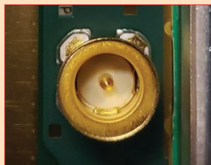
▲ Fig. 6 SMP male connector. Source: EJL Wireless Research LLC, January 2024.
