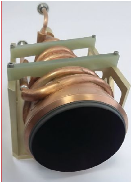
▲ Fig. 3 Thermal noise source with conical mmWave absorber. Source: TK Instruments Ltd.
