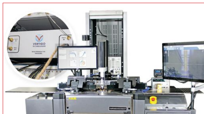
▲ Fig. 9 Active load-pull system with characterization software.
